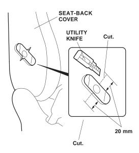
5. Using a felt-tip pen and tape measure, measure and mark the seat-back cover as shown. Push in on the mark, and confirm that the mark is centered over the hole in seat base.
