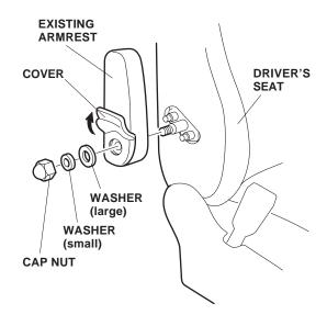
Remove the cap nut, small washer and large washer that secures the existing armrest, and remove the armrest.
