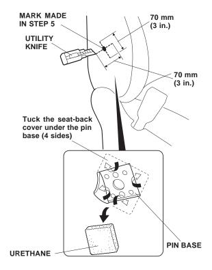
7. Get the new base from the kit, and position it on the pin base of the seat. Install the two socket bolts. Torque the socket bolts to 10-12 N·m (7-9 lbf·ft).
