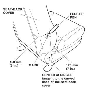
6. Using a utility knife, make two 70 mm (3 in.) cuts in the seat-back cover through the mark at right angle to each other as shown. Using these 70 mm (3 in.) cuts as a guide, cut out the marked area from the seat urethane to expose the seat base.
